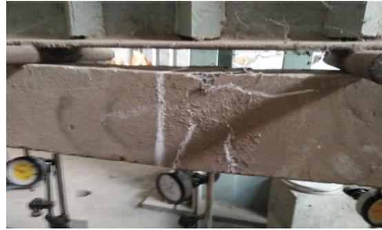
Figure 6: Failure of Beam 1
