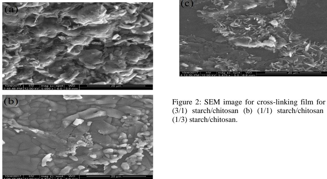
Figure 2: SEM image for cross-linking film for (a) (3/1) starch/chitosan (b) (1/1) starch/chitosan (c) (1/3) starch/chitosan.
