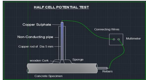
**Fig. 4. Half-cell potential test**
