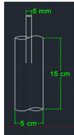
Fig. 1: concrete specimen
