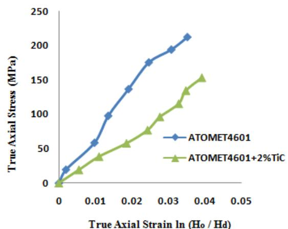
Fig.1. Plot of true axial stress versus true axial strain
