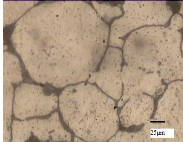
Fig. 6d: Microstructure of ATOMET4601 +2%TiC
