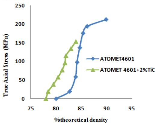
Fig.3. Plot of true axial stress versus % theoretical density
