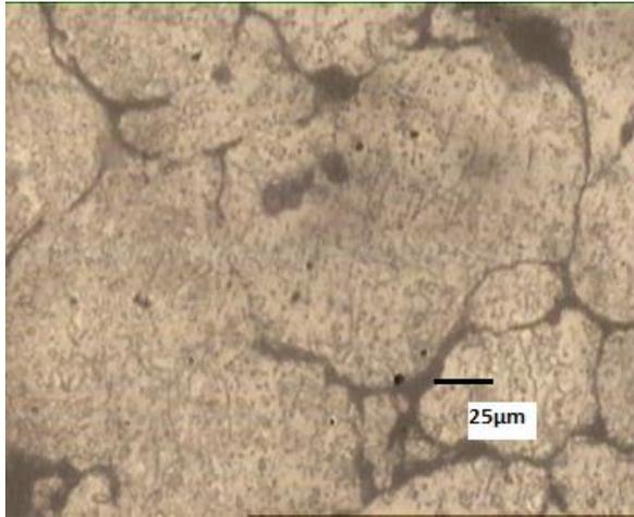
Fig. 6a: Microstructure of as sintered ATOMET4601
