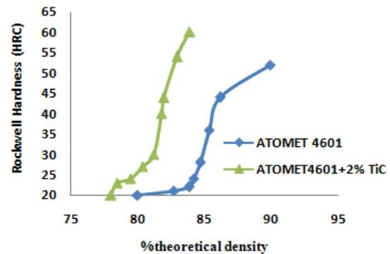
Fig.5. Plot of Rockwell hardness versus % theoretical density
