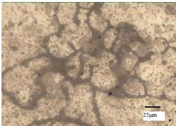
Fig. 6c: Microstructure of densified ATOMET4601
