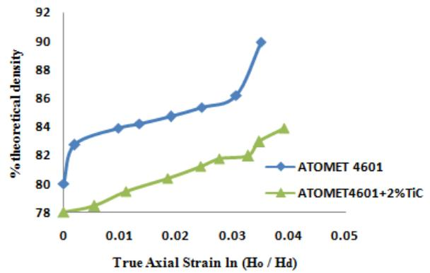
Fig.4. Plot of % theoretical density versus true axial strain
