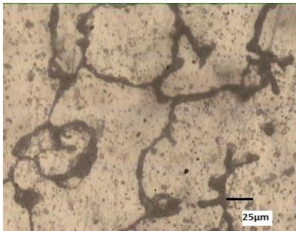
Fig. 6b: Microstructure of as sintered ATOMET4601 +2%TiC
