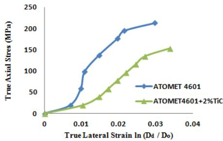
Fig.2. Plot of true axial stress versus true lateral strain
